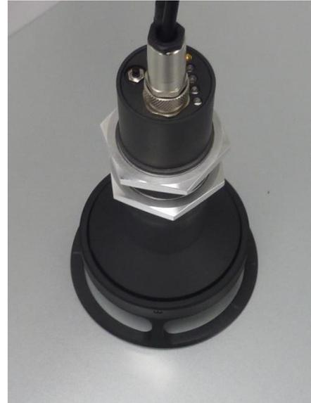
Offline attachment for laboratory measurements
